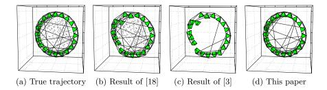
Fig. 3: Camera Pose registration problem results, a cone represents a camera pose, a black line is an inlier measurement and a gray dashed line is an outlier
