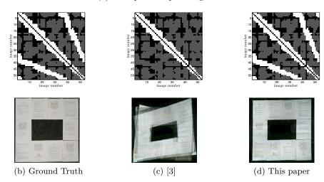
Fig. 4: Image mosaicking: in the labeling matrices a white pixel is an inlier, a black pixel corresponds to an unavailable measurement, a gray pixel corresponds to an outlier. Observe that our labeling inlier/outlier is perfect (see 4d).
