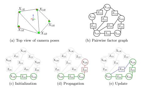
Fig. 1: Illustration of an outlier free consistent pose registration problem (Lie group SE(3)): (a) a cone represents a camera (global motion) and a link between two cones indicates that a relative motion measurement is available. (b)-(e) please see explanations in section 4.1
